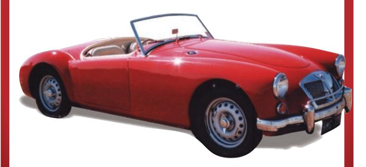
The 1600 MKII deLuxe was built using the last of the unused Twin Cam chassis. Like the Twin Cam, it has four wheel Dunlop disc brakes and disc wheels, but it has the 1622cc pushrod engine. This car is one of only 290 1600 MKII deLuxes built.
